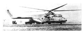
Figure 6-58. Mi-6 HOOK. This heavy-duty helicopter provides lift for 65 troops and about 16.5 tons of cargo. The short stub-wings are a distinctive feature.
